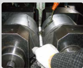
전조로링 (CYLINDRICAL THREAD ROLLING)
